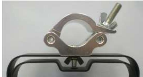
Regardless of the rigging option you choose for your MICROH LED COB100 PAR/RGBWA wash fixture, always be sure to secure your fixture with a safety cable. The fixture provides a built-in rigging point for a safety cable on the hanging bracket as illustrated above. Be sure to only use the designated rigging point for the safety cable and never secure a safety cable to a carrying handle.
